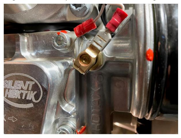
In order to avoid loose contacts and bad connections in the plug connections on the oil and water temperature sensors of the Rotax engine, I made a small clamp connection, which, like a pole clamp on a car battery, is pushed onto the cylindrical T-shaped sensor contacts of the temperature sensors and clamped with a screw.
